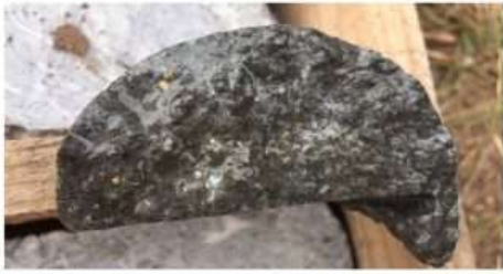
Visible gold in drill core from ATO-299
