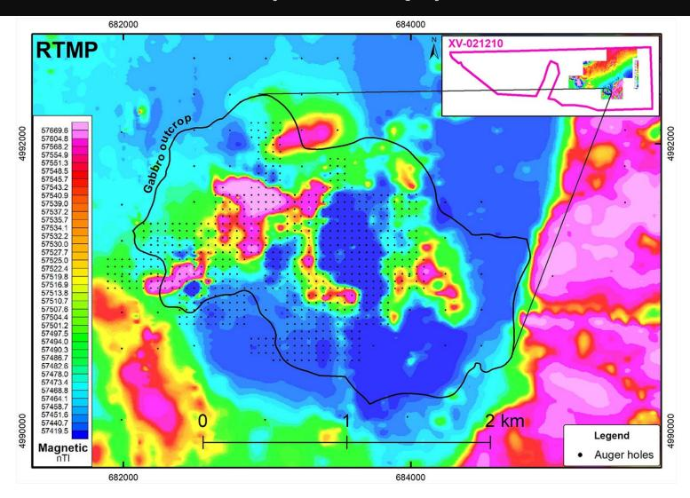
Ground Magnetic Geophysical survey results at the Victory Discovery.
